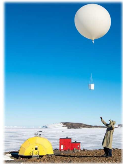
An ozone sonde being released at Davis station, Antarctica. (Photo: Barry Becker)
